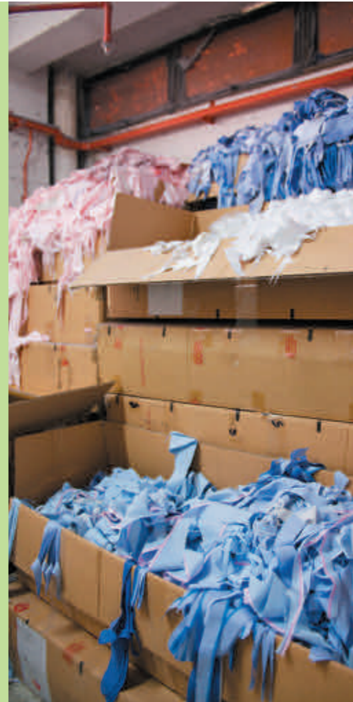
We collect remnants from the production floor and categorize remnants by colour. A baler machine is used to press remnants into a regular shape to facilitate transportation.
