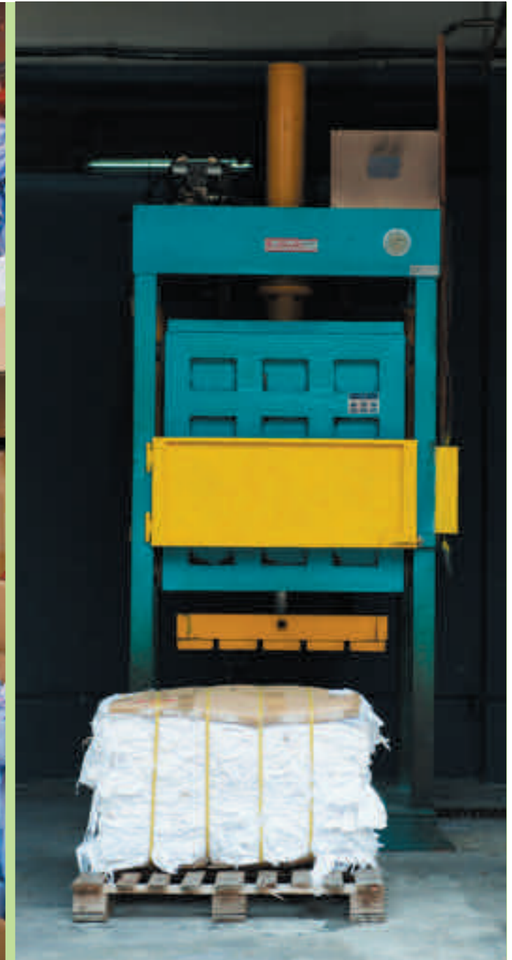
We collect remnants from the production floor and categorize remnants by colour. A baler machine is used to press remnants into a regular shape to facilitate transportation.
